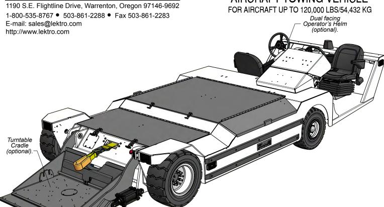
AP8850SDA-AL-100 FEATURES: Vehicle Drive: 45.3 HP/33.8 kW, 72 VDC Traction Motor mated with Auburn/Dana 44 Differential. Limited Slip Differential, optional.
